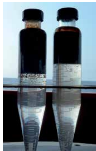
Result of a bottle test carried out on site
