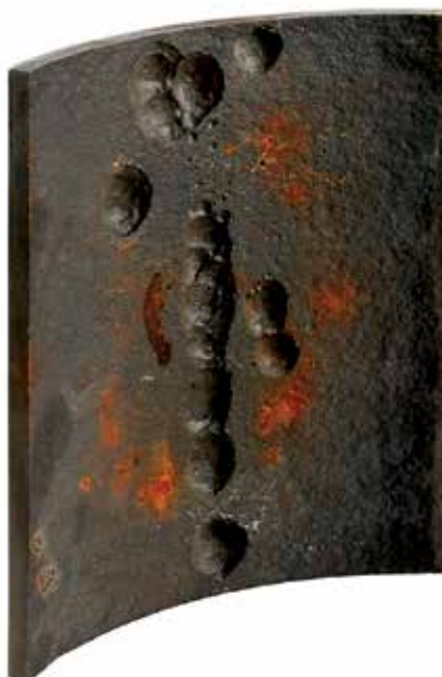
Cratering due to the presence of SRB/TRB
