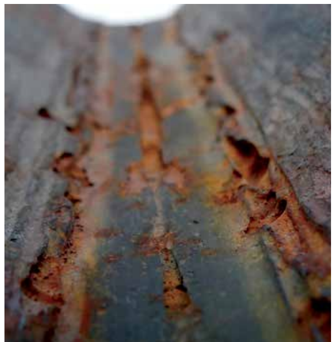
Cross-section of a carbon steel piece with various types of visible corrosion.
